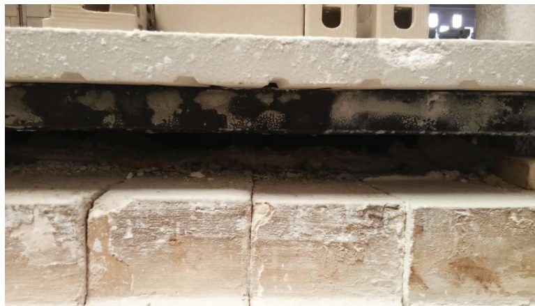
Figure 34: Low thermal mass in kiln car
