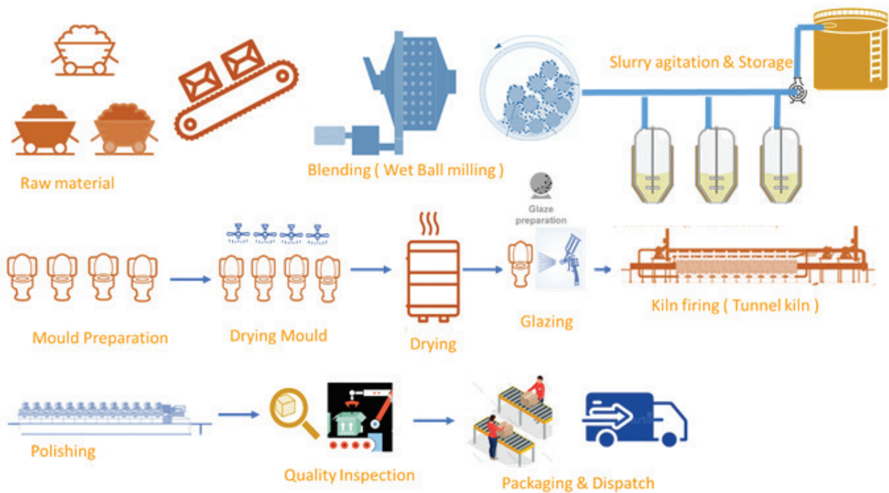
Figure 13: Ceramic Sanitaryware Manufacturing Process Flow
