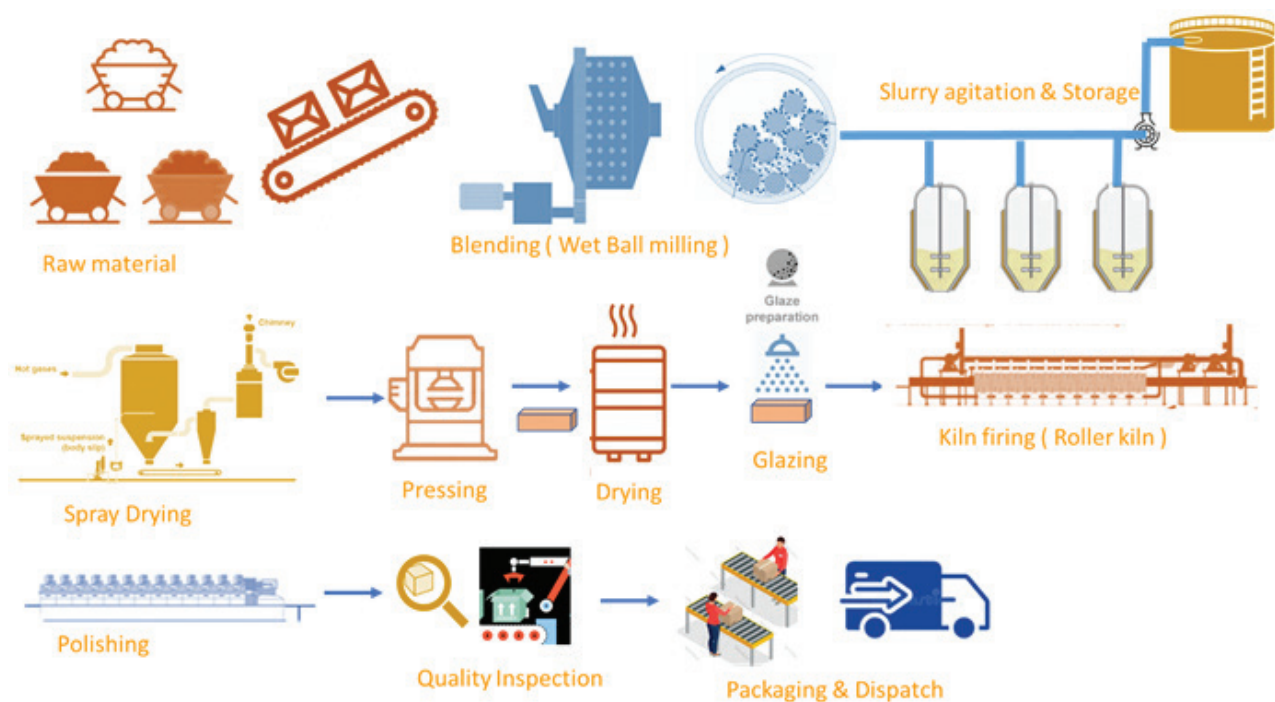
Figure 4: Ceramic Tile Manufacturing Process Flow
